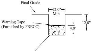
Conduit must be encased in concrete with 4 inches of cover
